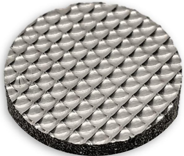
Figure 2: Near-final contour production of highly structured surfaces
