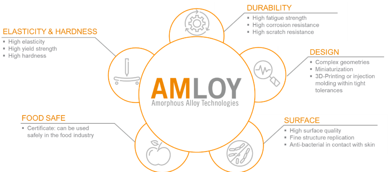
Figure 3: Advantages of amorphous metals in the field of high-performance grippers
