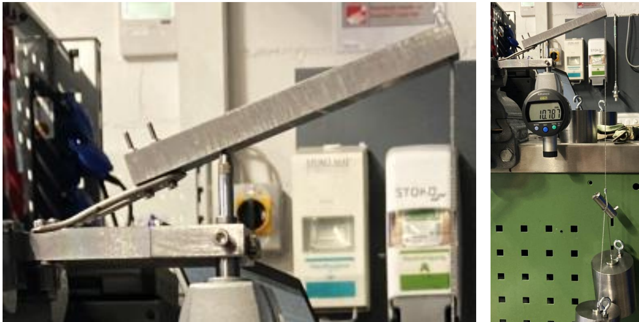
Figure 3: Experimental setup for the comparative measurement of TiGr2 and AMLOY ZR02 LCP's
